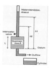
$$\ln \left(\frac{h_1}{h_2}\right) = \frac{kA}{aL} t \Rightarrow k = \frac{aL}{At} \ln \left(\frac{h_1}{h_2}\right)$$
