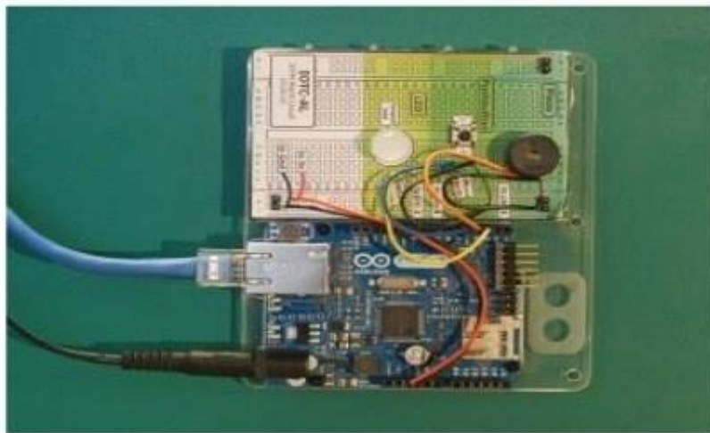
Fig: An Arduino Ethernet board, plugged in, wired up to a circuit and ready for use.
