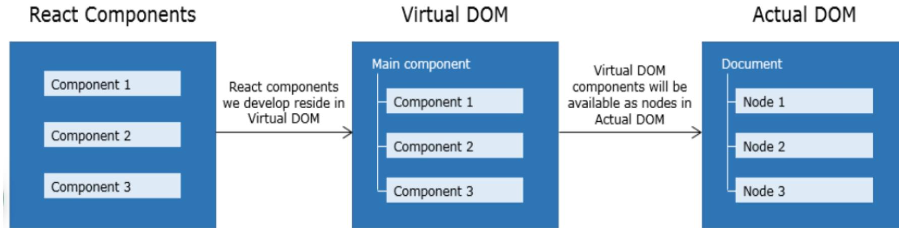
Virtual DOM is an abstraction of actual DOM, where components are the nodes. The virtual DOM can be programmatically modified by updating components. These updates are internally handled by React and in turn updated in actual DOM.
